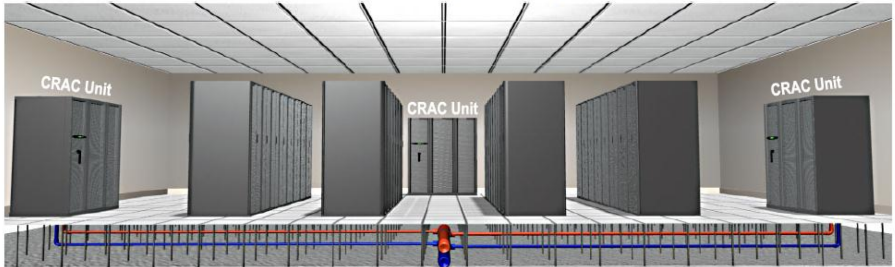
Figure 1 – Traditional underfloor chilled water piping installation with branches to different air conditioners using multiple fittings
