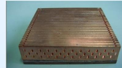
Type IV: Heat sink with loose vortex generator: The enhancements of this category are still vortex generators or dimple/protrusion structure but with sparse arrangement of vortex generator.
