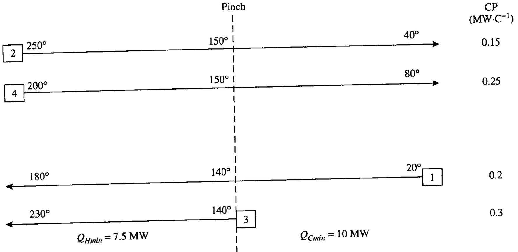
The grid diagram for the data from the Table 16.2.
