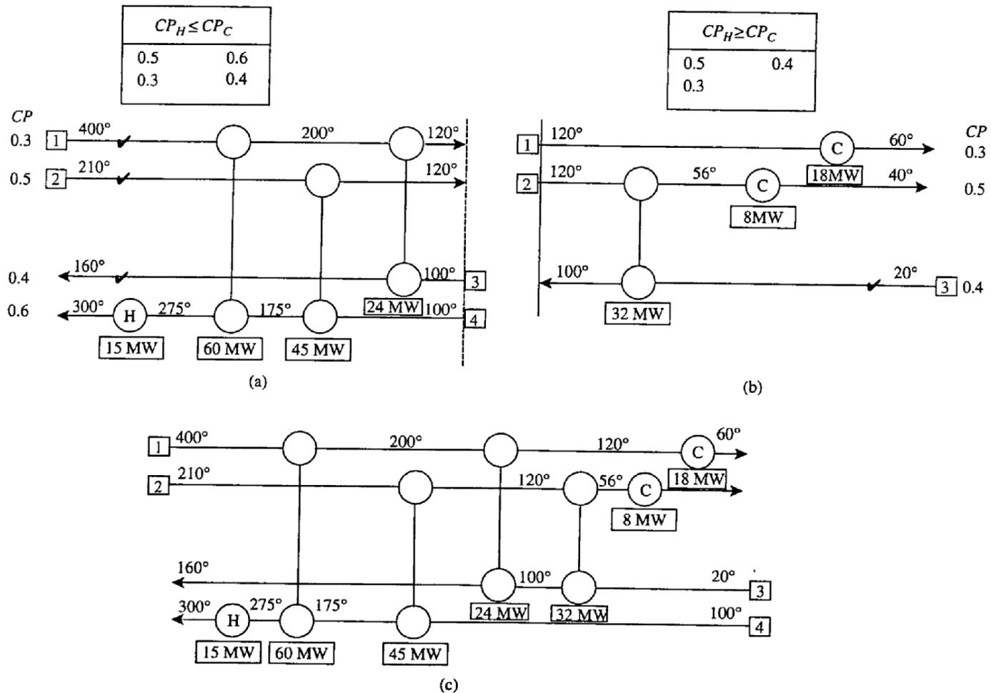
Figure 18.8 Maximum energy recovery design for Example 18.1.
