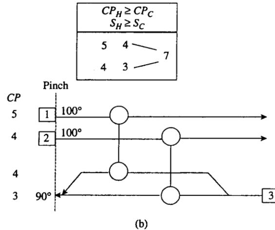
**Figure 18.15** The CP in equality rules can necessitate stream splitting below the pinch.
