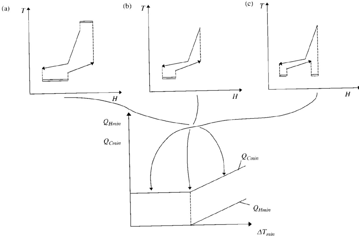
As  $\Delta T_{min}$  is varied, some problems require only cold utility below a threshold value.
