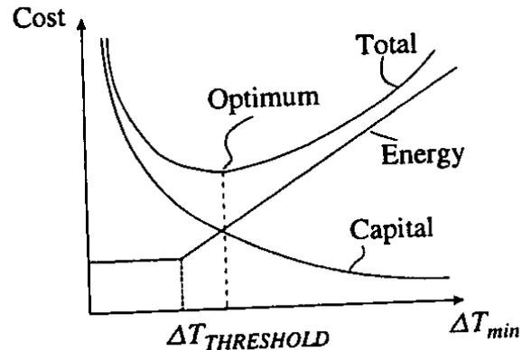
(b) The capital - energy trade-off can lead to an optimum above  $\Delta T_{THRESHOLD}$
