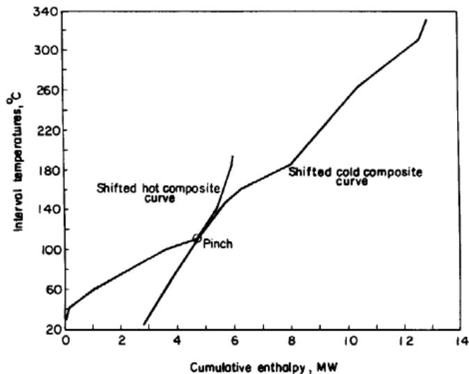
Sketch 6.2 Shifted composite curves (interval temperature basis)
