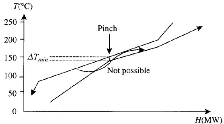
(c) Heat transfer from below to above the pinch is not possible without violating  $\Delta T_{min}$ .
