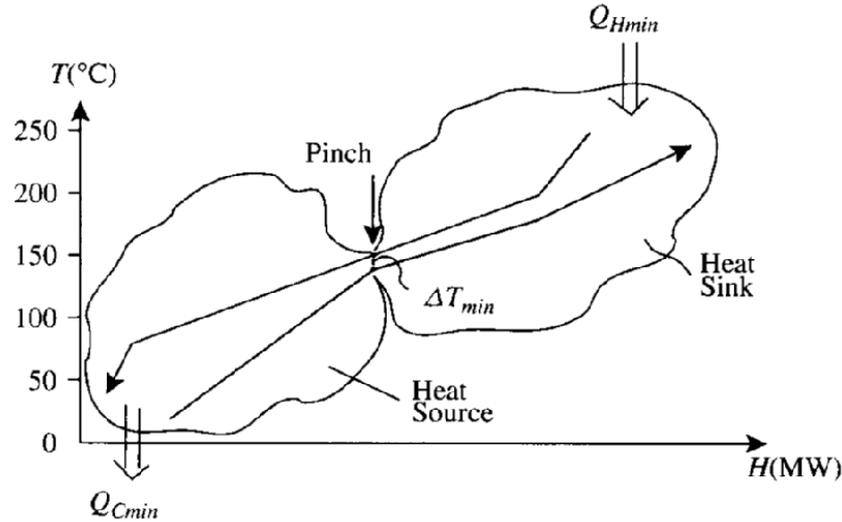
(a) The pinch divides the process into a heat source and a heat sink.
