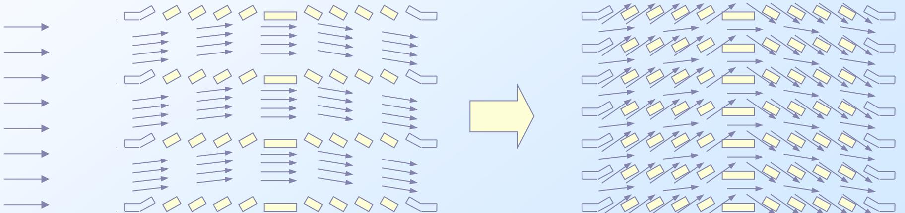
**SCHEMATIC OF DUCT FLOW VS. FIN-DIRECTED FLOW FOR LOUVER FIN GEOMETRY AT SMALLER AND LARGER FLOW VELOCITIES. (Yang et al. IJHMT, 2007)**
