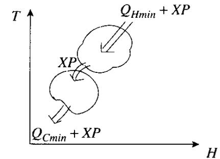
(a) Process-process heat transfer across the pinch.
