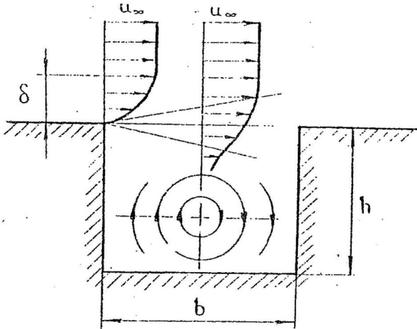
Fig. 1. Model of flow in an isolated rectangular pit [2] in a wall.
