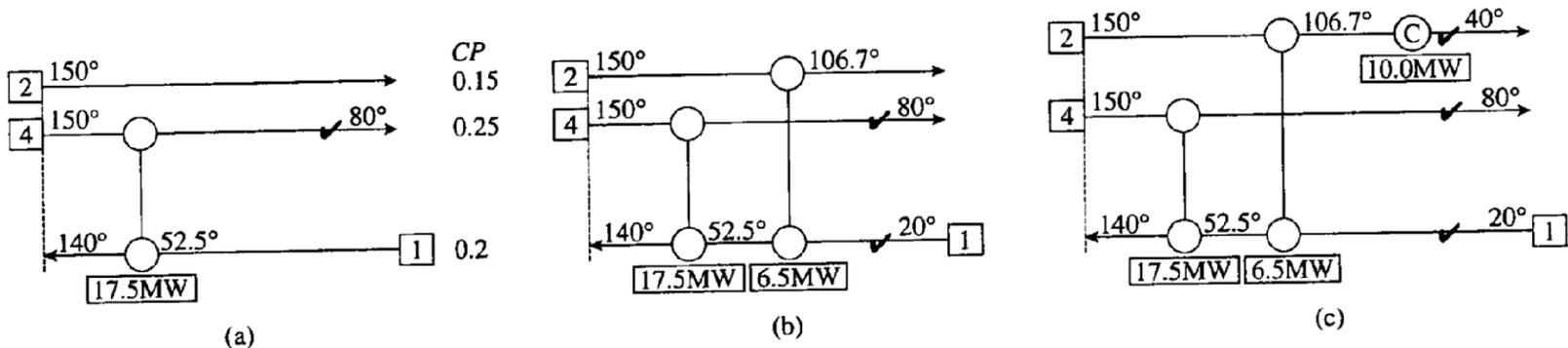
Figure 18.6 Sizing the units below the pinch using the tick-off heuristic.
