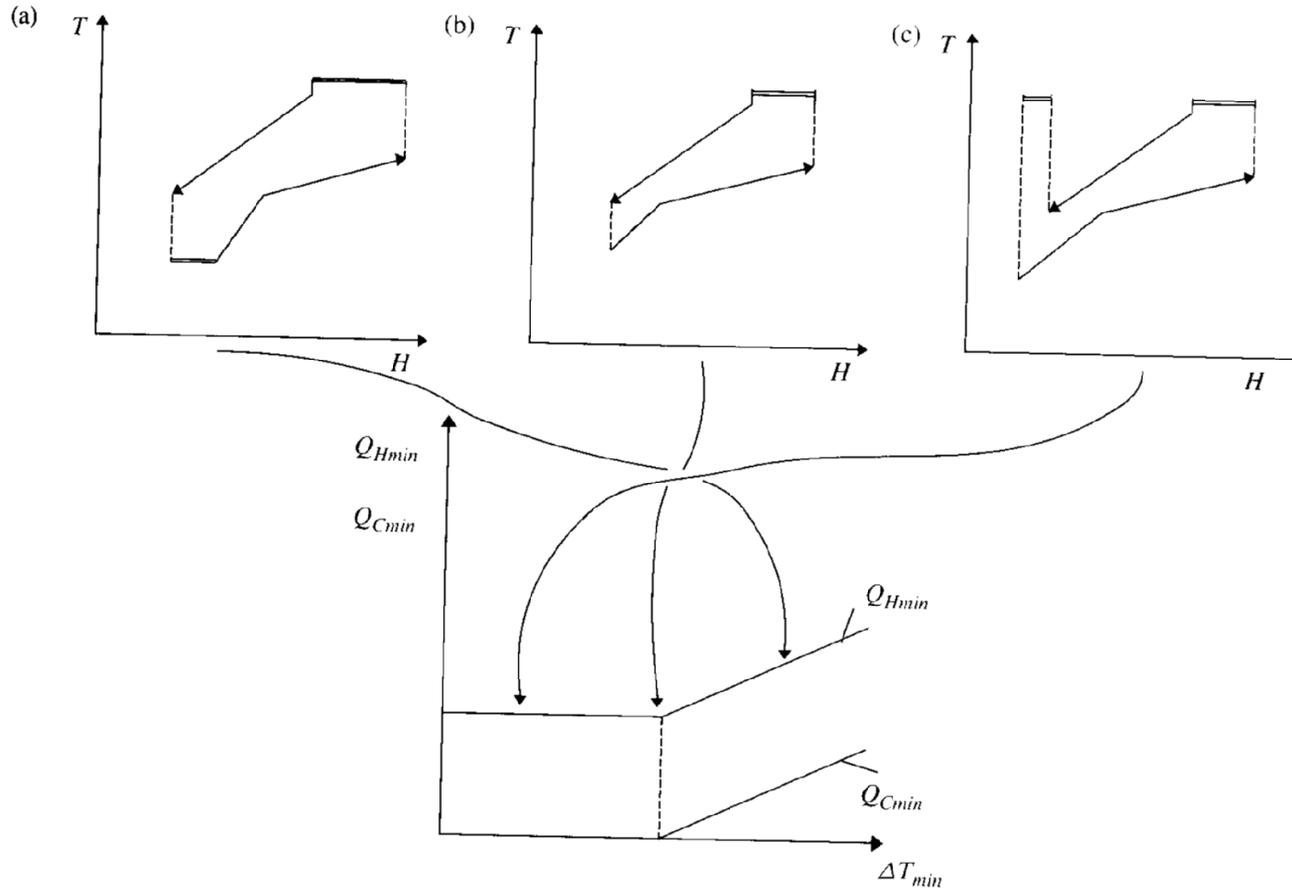
In some threshold problems, only hot utility is required below the threshold value of  $\Delta T_{min}$ .
