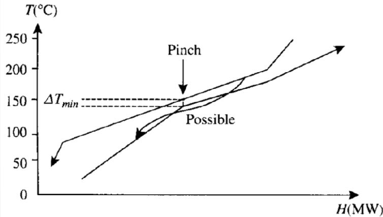
(b) Heat transfer from above the pinch to below the pinch is possible.
