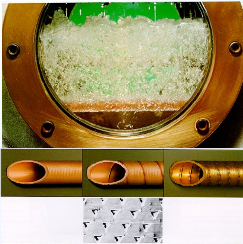
Shell side boiling
