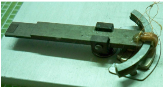
Fig. 5. (Color online) Fabricated “seesaw-shaped” VCM actuator.
